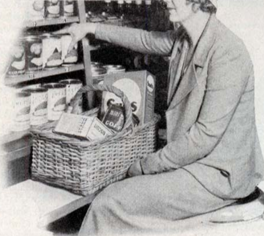
From the moving shelves of the self-service grocery store shown above, the purchaser selects goods as they pass on endless chain
